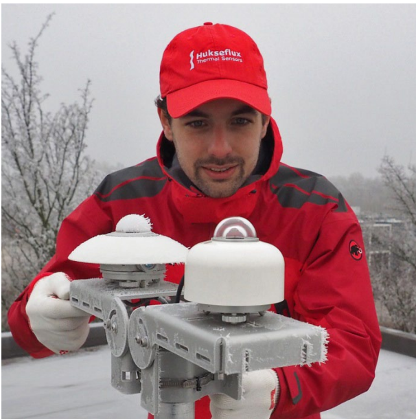
Figure 3 frost and dew deposition: clear difference between a non-heated pyranometer (back) versus SR30 (front)
