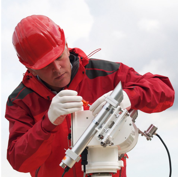
Figure 1 installing a DR01 first class pyrliometer
