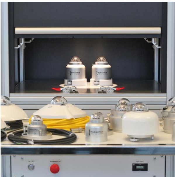
Figure 1 Calibration of all major pyranometer brands.
