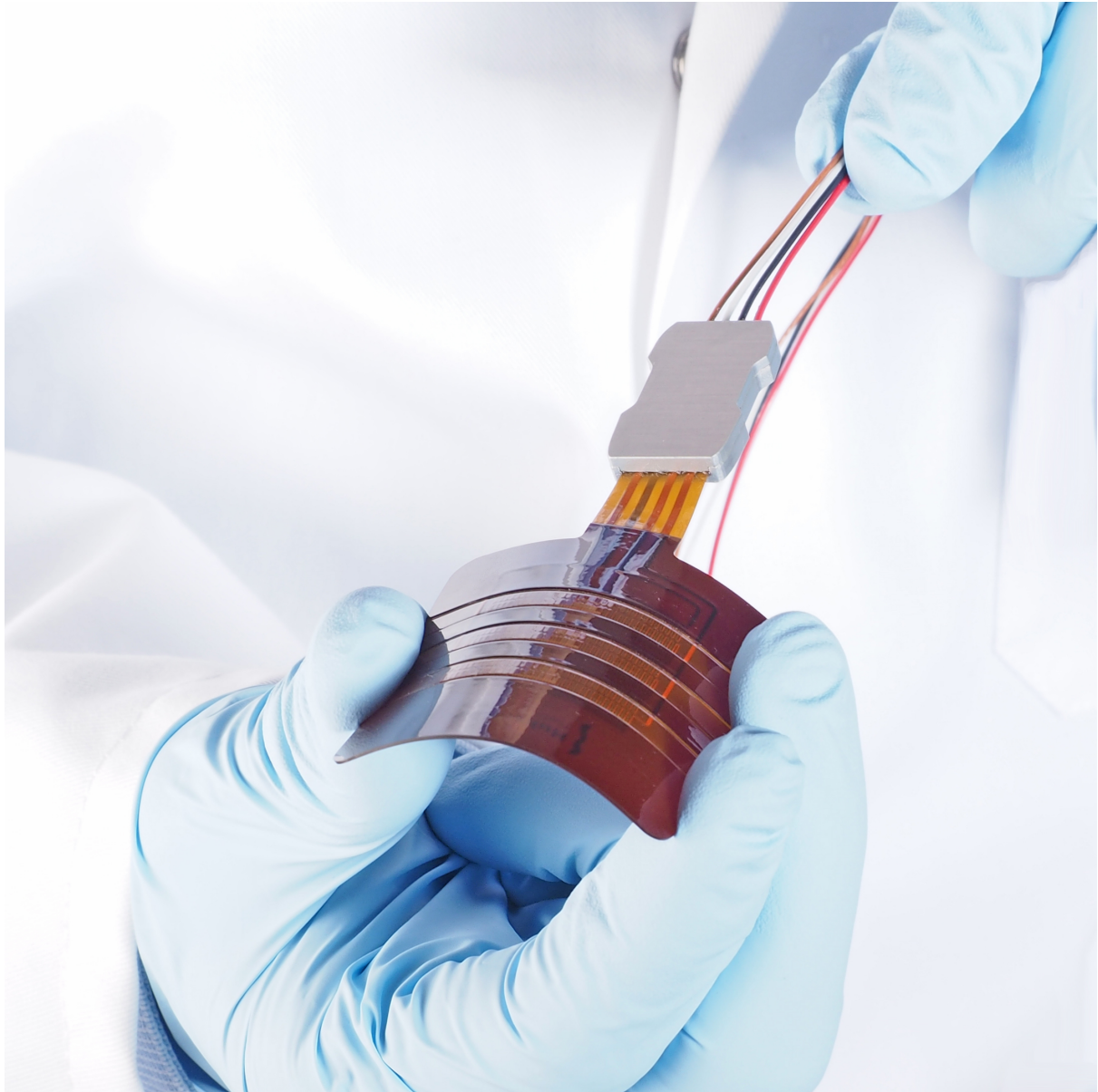
Figure 5.2.1 Bending direction of FHF01. Bending the FHF01 in this direction minimizes the strain on the sensor and improves the measurement result
