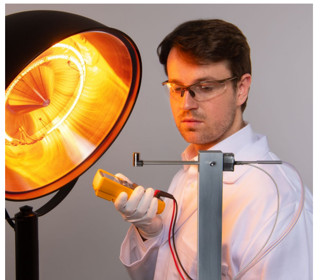
Figure 2 SBG04 is the sensor of choice for cone calorimeter calibration.
