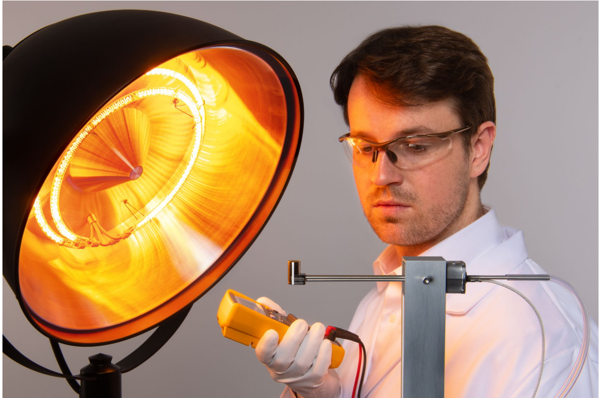
Figure 1.4 SBG04 is the sensor of choice as calibration reference standard for cone calorimeter test equipment, but may also be used for other purposes.
