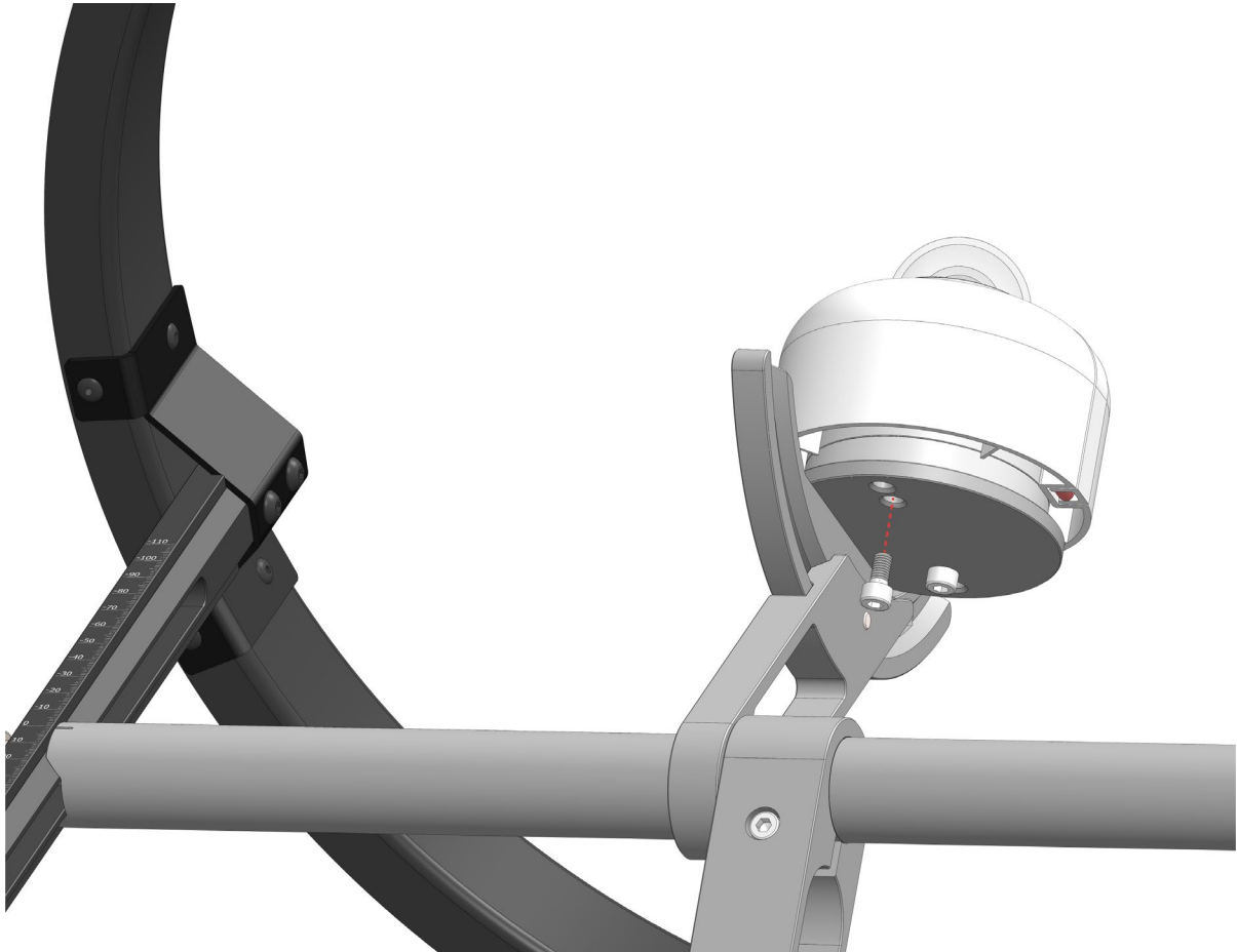
Figure 5.4.3.1.1 Mounting an SR15 pyranometer on SHR02
