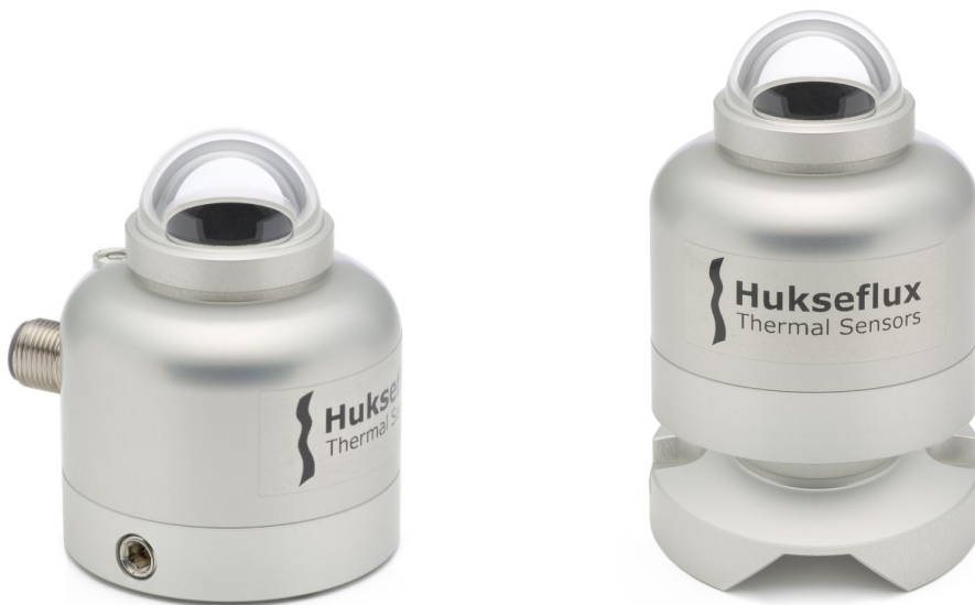
Figure 0.3 On the left SR05-D1A3-PV pyranometer with bubble level and M12-A cable connector in its standard configuration (3 metre cable standard included); on the right SR05 with optional ball levelling, for easy mounting and levelling on (non-)horizontal surfaces (included mounting bolts not displayed)
