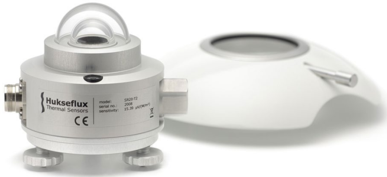
Figure 0.1 SR20 Class A pyranometer with its sun screen removed.
