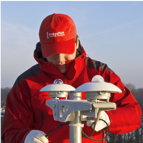
Figure 2 Frost deposition: clear difference between SR25 (left), versus a non-heated pyranometer without sapphire dome (right).
