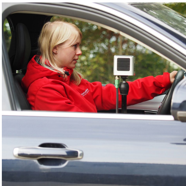
Figure 4 TCOM01 applied in car passenger comfort testing
