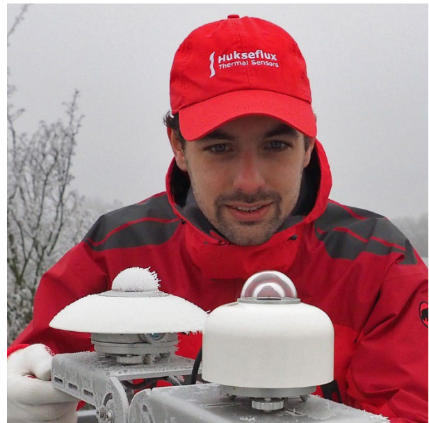
Figure 2 A typical problem in freezing conditions: ice accumulation on the dome surface of a traditional pyranometer reduces data availability. SR30 in front is heated.
