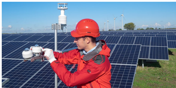
Figure 2 Two SR30 Class A pyranometers measuring GHI (Global Horizontal Irradiance) and POA (Plane of Array) in a PV performance monitoring system.
