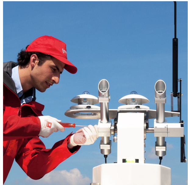
Figure 2 Typical reference measurement station with a solar tracker, pyr heliometers model DR02 and pyranometers model SR20.
