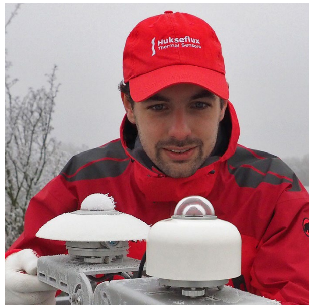
Figure 1 Frost and dew deposition: clear difference between a non-heated pyranometer (back) and SR30 with heating.
