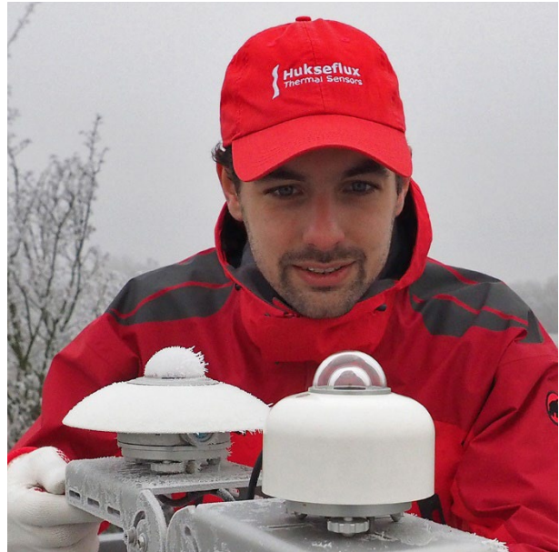
Figure 3 Hukseflux model SR30 (at the front) is the first heated pyranometer, compliant with the requirements of IEC 61724-1 for Class A monitoring systems. It mitigates dew and frost as seen on the non-heated pyranometer at the back: dew and frost deposition on the pyranometer dome reduce data availability and accuracy.
