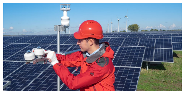
Figure 2 PV system performance monitoring with pyranometers measuring GHI and POA.
