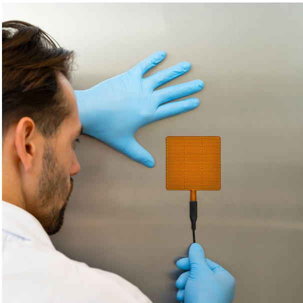
Figure 1 FHF05SC-85X85 Heat flux sensor mounted on a wall, using silicone glue (NR 5 in table 1). NOTE: sensor optical properties do not match those of the metal wall it will later be covered with a metal cover so that optical properties match (NR 4 in table 3).
