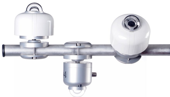
Figure 1 In PV system performance monitoring users typically employ Plane of Array (POA) on the right, Global Horizontal Irradiance (GHI), on the left, and increasingly also Reflected Irradiance (RI), in the middle.
