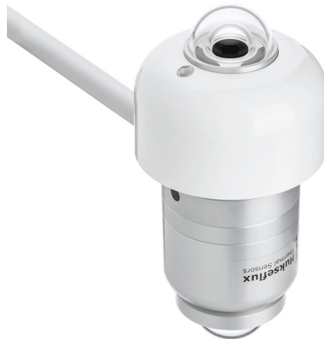
Figure 2 2 x SR30 spectrally flat Class A (secondary standard) pyranometer connected to a fixture plus rod, together forming an albedometer. The downfacing pyranometer is equipped with a glare screen to block solar radiation entering the lower detector at low solar angles (150 ° instead of 180 ° full field of view angle).
