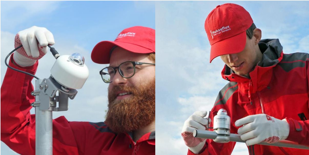
Figure 4 a) SR30 mounted using a PMF01 bracket on a vertical pole in tilted orientation, b) SR05 with ball levelling and tube mount installed on a horizontal tube.
