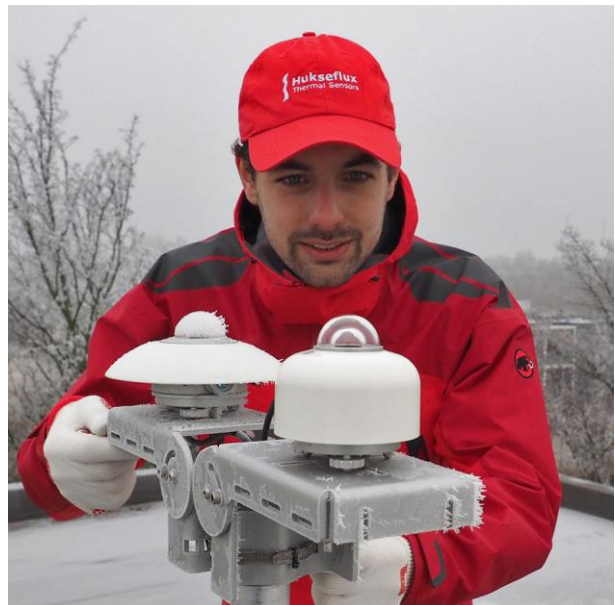
Figure 1 A typical problem in freezing conditions: ice accumulation on the pyranometer dome surface reduces data availability. At the front, the new SR30 pyranometer design with recirculating ventilation.
