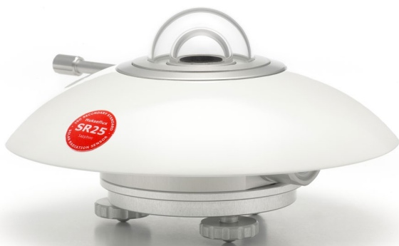
Figure 2 Example of a Hukseflux spectrally flat Class A pyranometer, model SR25, with a sapphire outer dome. This model is recommended for research grade diffuse radiation measurement. Output is either analogue millivolt or digital via Modbus RTU over RS-485 and analogue 4-20 mA (current loop).
