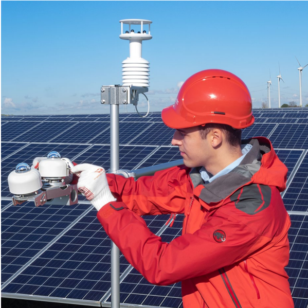
Figure 1 SR30 pyranometers, our most popular solution for PV system performance monitoring according to IEC 61724-1 class A.
