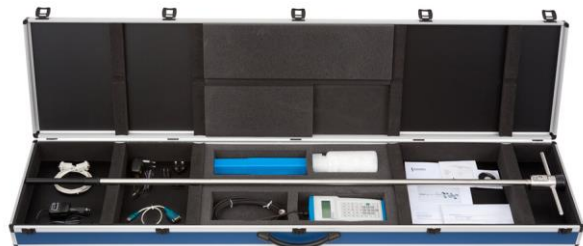
Figure 4 The complete and robust FTN02 measuring system including the 1.4 m long lance LN02
