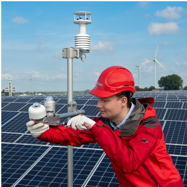
Figure 2 Typical use of pyranometers at PV power plants. The above picture shows two SR200-D1 pyranometers, one tilted for Plane of Array (POA) measurement, and another mounted horizontally for Global Horizontal Irradiance (GHI) measurement.
